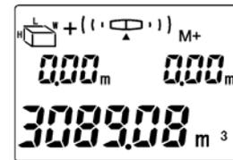
Note: If continuously press the  $\boxed{+/-}$  key for 2 times, the addition operation will be canceled and the icon  $\boxed{+/-}$  will disappear (Press  $\boxed{+/-}$  key shortly for one time will enter into addition, Press  $\boxed{+/-}$  key shortly for two times will cancel the operation. Then press again will toggle back and forth between: add----cancel----add).
