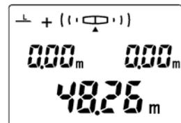
Note: If continuously press the  $\boxed{+/\equiv}$  key for 2 times, the addition operation will be canceled, all the anterior computation result will clear away.
